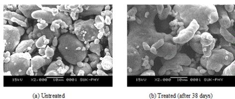
**Figure 3:** Scanning electron microscope pictures of untreated and powders treated after 38 days showing a rounding, and coarsening of particles due to joining of several particles at inter particle boundaries.
