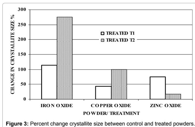
Figure 3: Percent change crystallite size between control and treated powders.
