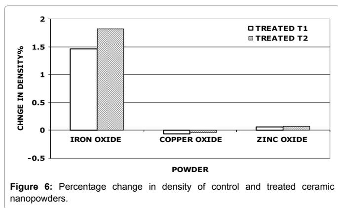
Figure 6: Percentage change in density of control and treated ceramic nanopowders.
