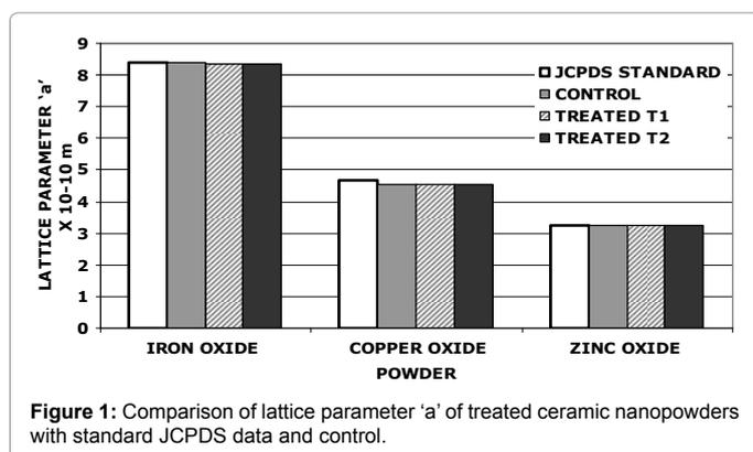
Figure 1: Comparison of lattice parameter 'a' of treated ceramic nanopowders with standard JCPDS data and control.
