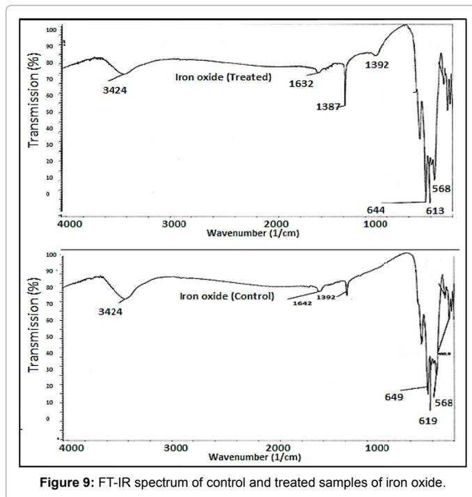
Figure 9: FT-IR spectrum of control and treated samples of iron oxide.
