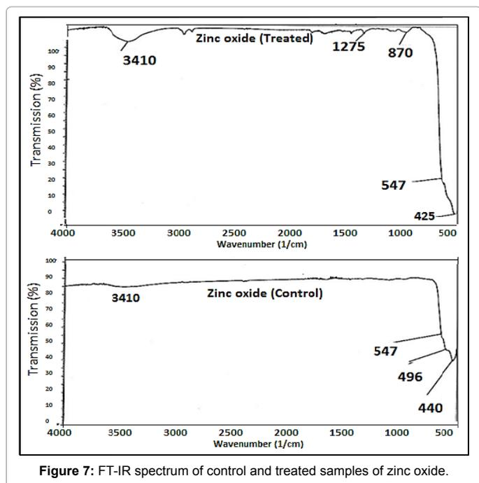
Figure 7: FT-IR spectrum of control and treated samples of zinc oxide.
