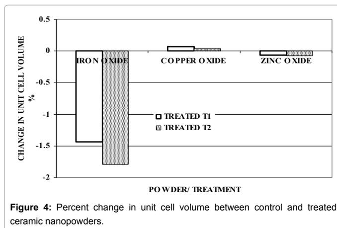
Figure 4: Percent change in unit cell volume between control and treated ceramic nanopowders.
