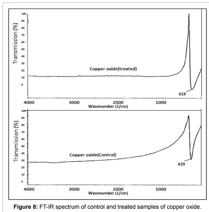
Figure 8: FT-IR spectrum of control and treated samples of copper oxide.
