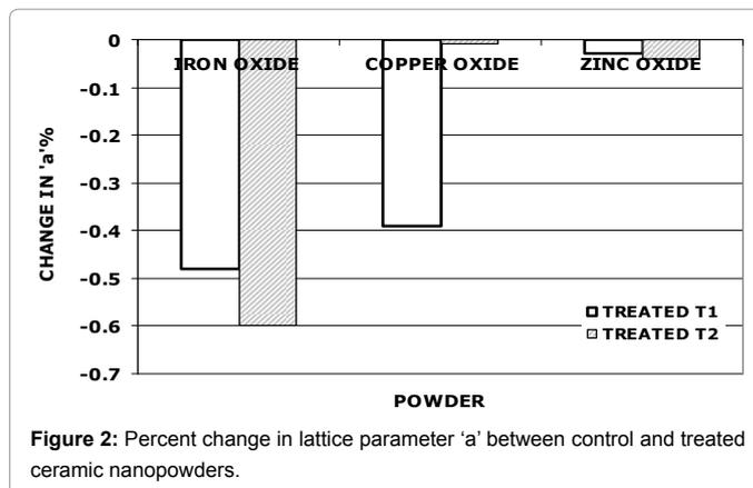
Figure 2: Percent change in lattice parameter 'a' between control and treated ceramic nanopowders.
