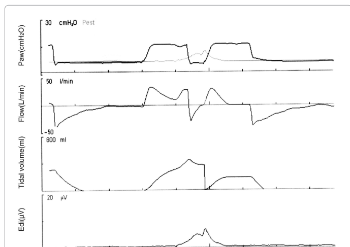
Figure 1: Traces are airway pressure, flow, tidal volume, an electrical activity of the diaphragm during mechanical ventilation in pressure control mode. Mechanical breath triggered neural effort and induced double cycling. (Paw=Airway pressure; EAdi=An electrical activity of the diaphragm).
